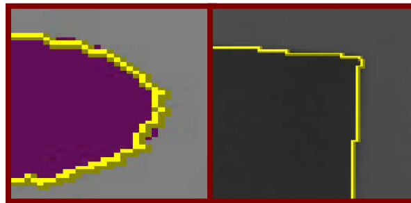
Figure 1. Noise and quantization (right) error in boundary extraction masks the local curvature
