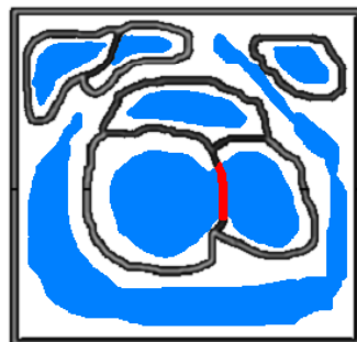
Forming dam(s) where water from two catchment basins meet.
