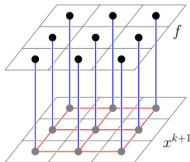
$$E_{k+1} = \sum_{e_{ij} \in E} \left( e^{-(x_i^k - x_j^k)^2} \right)^\alpha (x_i^{k+1} - x_j^{k+1})^2 + \lambda \sum_{v_i \in V} \left( e^{-(x_i^k - f_i)^2} \right)^\alpha (x_i^{k+1} - f_i)^2$$
