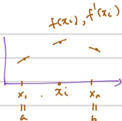
$$S(x) = S_i(x) \quad x \in [x_i, x_{i+1}] \quad i = 1, \dots, n-1$$
