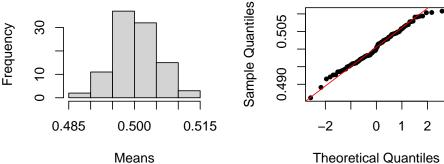
Again, it can be seen from histogram that data tends to symmetric with increase in 'n'. Also, from the QQ-Plot we can conclude that the data distribution is normal.
