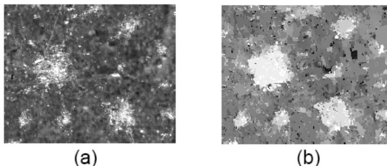
Fig.2: Subsample of (a) original SAR intensity data and (b) the corresponding GIS-aided segmentation result (Logarithmic mean values of backscattered intensity are assigned to each segment).
