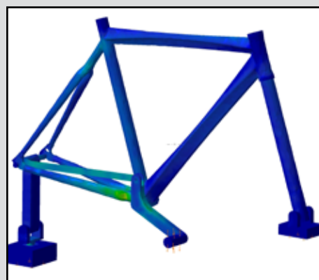
Typical FEA model for studying pedaling forces on the frame.
