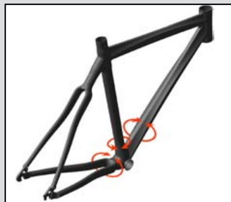
Twisting forces put on frame tubes during pedaling.
