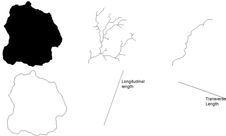
Basic measures for a basin, (a) basin area, (b) total channel length, (c) main channel length, (d) basin perimeter, (e) longitudinal length and (f) transverse length.
